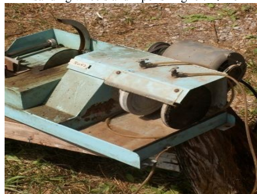
6 inch trim saw with two 6 inch grinding wheels. Motor runs $125.00
